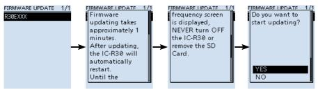
**TIP:** To check the firmware version after the updating, see "Checking the firmware version (p. 9-3)" for details.
