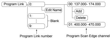
① When only one Program Scan Edge channel is entered, or there is no Programmed Scan Edge is left, "Add" is not displayed after pushing [QUICK].
