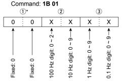
\*Not necessary when setting a frequency.
