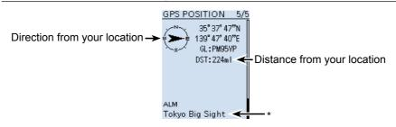
\* When a name is not entered in the GPS Memory channel, date and time are displayed instead of the name. You can change the GPS Memory or GPS Alarm on the GPS POSITION screen. (p. 5-5)
