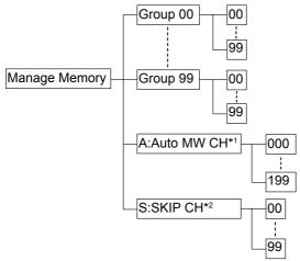
\*1 Automatically writes when a signal is received.
